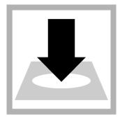
**8.** Insert the blank into the cell holder. Point the triangle mark on the sample cell away from the keypad.
