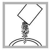
**3.** Add two DPD Total Chlorine Reagent Powder Pillows to the sample cell.
