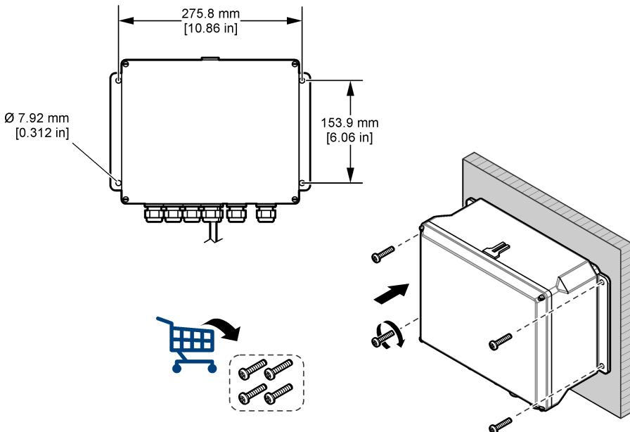
**Figure 3 Mounting locations on the sampler**
