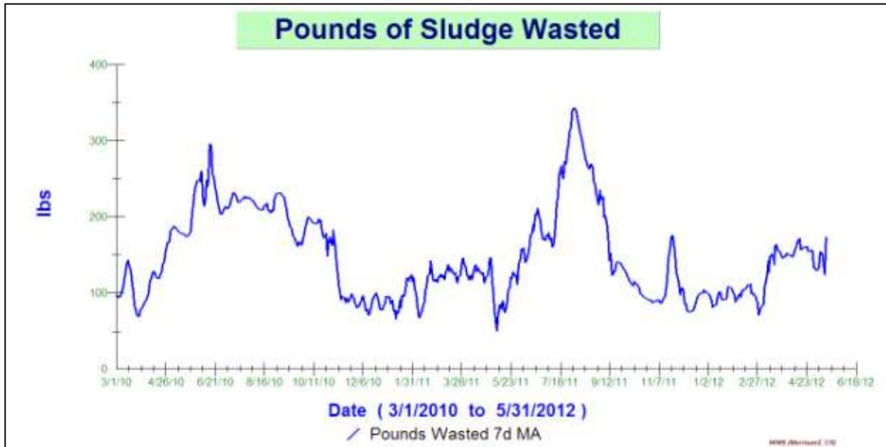
Other benefits that the staff have discovered include: reducing operator error (especially error between operators); reducing overwasting events which would fill the digester to capacity; being able to operate at a higher sludge age, which reduces the sludge yield; and creating a more consistent operation without large swings.
